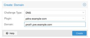
After configuring the desired domain(s) for a node and ensuring that the desired ACME account is selected, you can order your new certificate over the web interface. On success the interface will reload after 10
