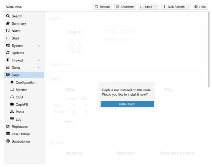
With Proxmox VE you have the benefit of an easy to use installation wizard for Ceph. Click on one of your cluster nodes and navigate to the Ceph section in the menu tree. If Ceph is not already installed, you will see a prompt offering to do so.
