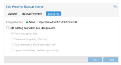
Optionally, you can configure client-side encryption with AES-256 in GCM mode. Encryption can be configured either via the web interface, or on the CLI with the <code>encryption-key</code> option (see above). The key will be saved in the file /etc/pve/priv/storage/<STORAGE-ID>.enc, which is only accessible by the root user.
