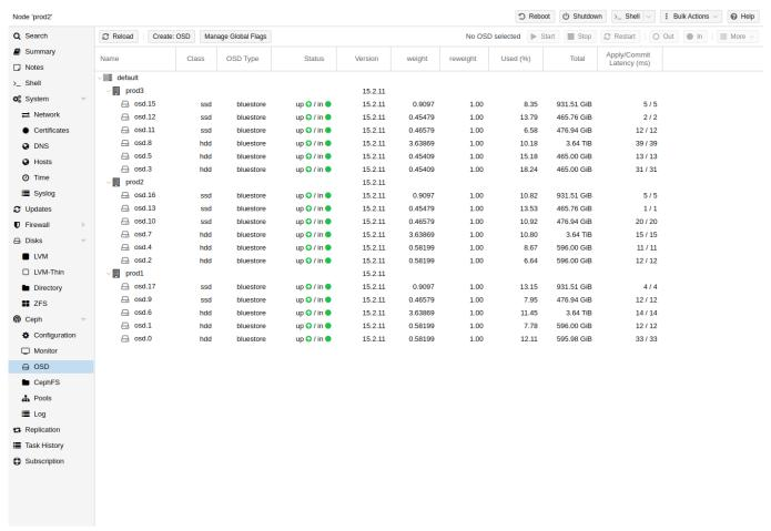
Ceph Object Storage Daemons store objects for Ceph over the network. It is recommended to use one OSD per physical disk.
