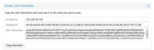
Log in to the web interface on an existing cluster node. Under Datacenter o Cluster, click the **Join Information** button at the top. Then, click on the button **Copy Information**. Alternatively, copy the string from the *Information* field manually.
