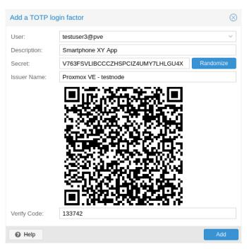
There is no server setup required. Simply install a TOTP app on your smartphone (for example, FreeOTP) and use the Proxmox Backup Server web interface to add a TOTP factor.
