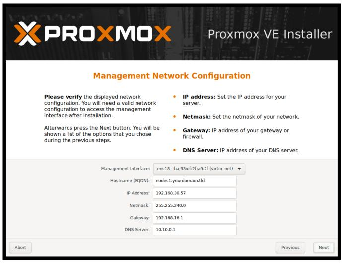
The last step is the network configuration. Network interfaces that are UP show a filled circle in front of their name in the drop down menu. Please note that during installation you can either use an IPv4 or IPv6 address, but not both. To configure a dual stack node, add additional IP addresses after the installation.
