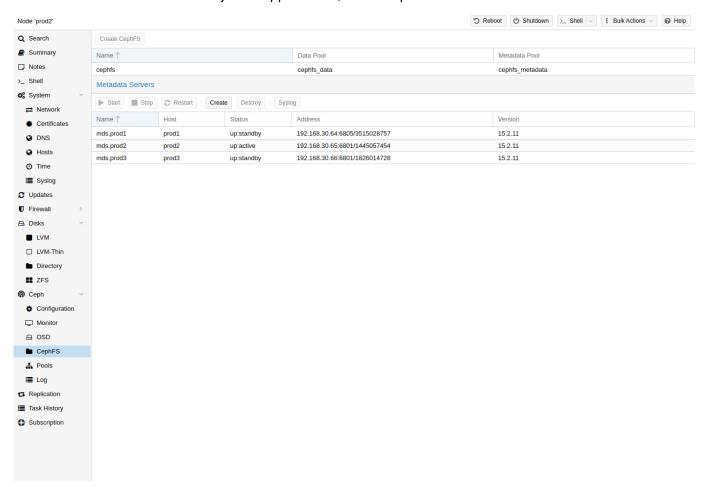
Proxmox VE supports both creating a hyper-converged CephFS and using an existing CephFS as storage to save backups, ISO files, and container templates.
