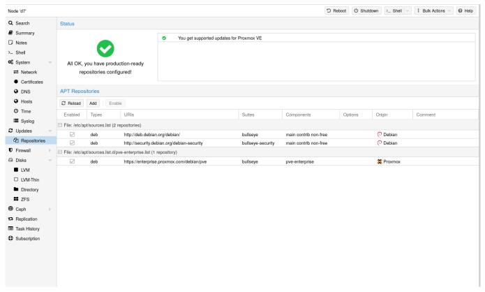
Since Proxmox VE 7, you can check the repository state in the web interface. The node summary panel shows a high level status overview, while the separate *Repository* panel shows in-depth status and list of all configured repositories.
