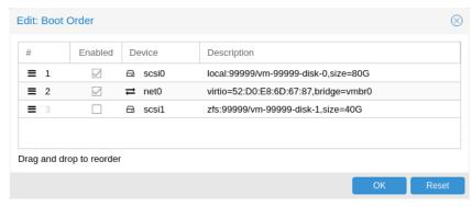
This way, the guest would first attempt to boot from the disk scsi0, if that fails, it would go on to attempt network boot from net0, and in case that fails too, finally attempt to boot from a passed through PCIe device (seen as disk in case of NVMe, otherwise tries to launch into an option ROM).
