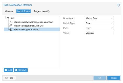
Notification matchers route notifications to notification targets based on their matching rules. These rules can match certain properties of a notification, such as the timestamp (match-calendar), the severity of the notification (match-severity) or metadata fields (match-field). If a notification is matched by a matcher, all targets configured for the matcher will receive the notification.
