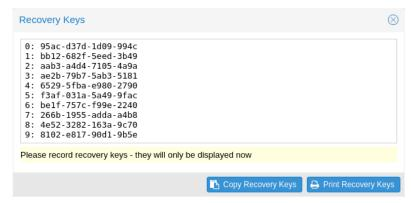
Recovery key codes do not need any preparation; you can simply create a set of recovery keys in the **Two** Factor panel under **Datacenter**  $\rightarrow$  **Permissions**  $\rightarrow$  **Two Factor**.
