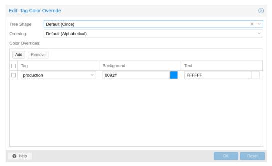
By default, the tag colors are derived from their text in a deterministic way. The color, shape in the resource tree, and case-sensitivity, as well as how tags are sorted, can be customized. This can be done via the web interface under Datacenter o Options o Tag Style Override. Alternatively, this can be done via the CLI. For example:
