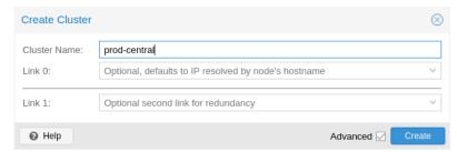
Under Datacenter o Cluster, click on **Create Cluster**. Enter the cluster name and select a network connection from the drop-down list to serve as the main cluster network (Link 0). It defaults to the IP resolved via the node's hostname.
