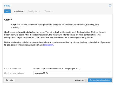
After finishing the installation step, you will need to create a configuration. This step is only needed once per cluster, as this configuration is distributed automatically to all remaining cluster members through Proxmox VE's clustered configuration file system (pmxcfs).
